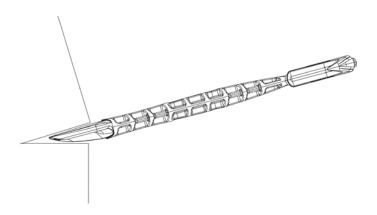
In the head of the axe blade there is a spade-shaped hole designed primarily for **right angle prying** with a second Paratech Crash Axe (or other Paratech Forcible Entry Tool) when extra leverage is required. This hole may also be used for attaching rope for use as a grappling hook or as a notch for storing the tool.
