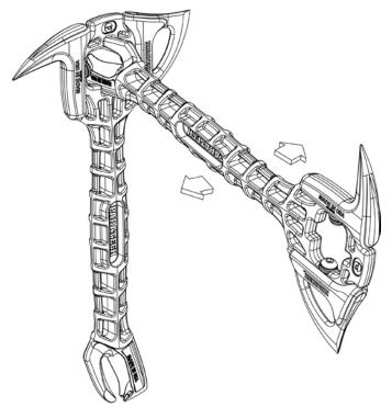
Minimal maintenance for the Paratech Crash Axe is required. To remove debris, wash with water and mild soap. Dry thoroughly. The Topcut blade and Pike can all be sharpened as needed or replaced with a single 3/16" hex key. There is no plating to worry about chipping since the tool bits are stainless steel and electropolished.\*
