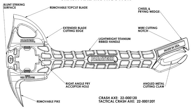
The Paratech Crash Axe is designed to be an ergonomic, lightweight, wearable (using available holster) multi-purpose tool system that can be employed without preparation and used for forcible entry, extraction, and rescue. The Paratech Crash Axe complies with SAE International Aerospace Standard AS5402 and NTSB Crash Axe requirements.
