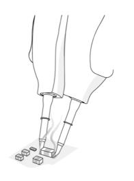
Once in position, press and hold the pedal to perform the soldering
